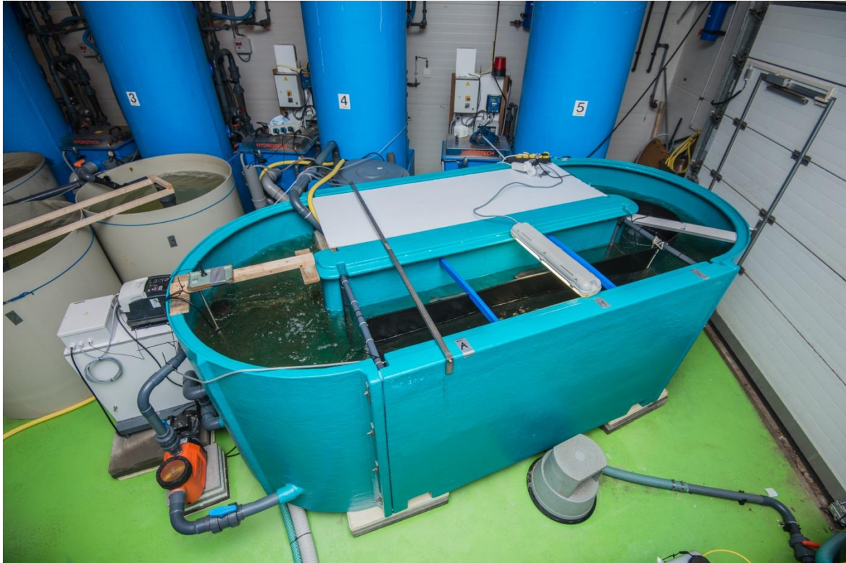
Figure 1. The swim-flume. Treated eels were housed in the swimming compartment (compartment where the water current arrives through the outer curve). During the experiment, the flume was covered with thick black foil to shield the eels from exogenous light and artificial light was only provided during FW-migration.
